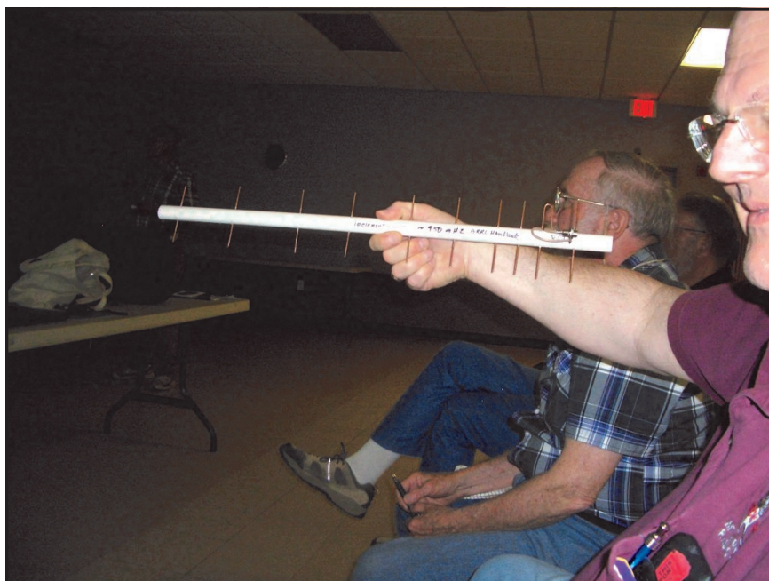
Here's a 10 element PVC pipe and 12 Ga. wire yagi that works well with the SDR dongle.
